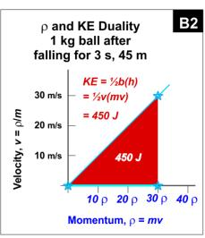
At the bottom of the swing, Ball-1 has a velocity of 30 m/s and a momentum of 30  $\rho$ . The energy implications can be visualized by converting the impulse-velocity graphs into line graphs. Using the impulse and energy equations a combined line graph for the potential energy acquisition of a 1 kg object can be made, Illustration C1:
